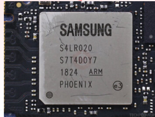
Samsung Phoenix Controller features 5 ARM Cortex-R7 cores
