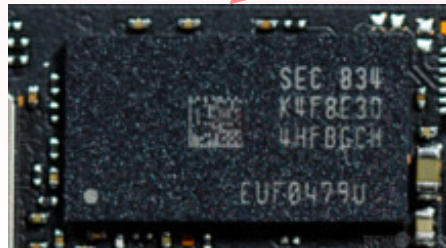
Samsung LPDDR4-1866 DRAM features a 1 GB capacity
